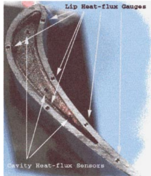
Fig. 3 Photograph of cavity and lip heat-flux gauges
