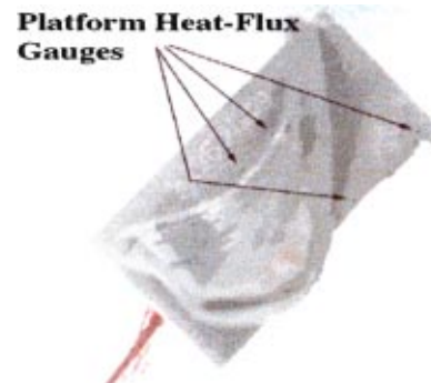
Fig. 4 Photograph of platform heat-flux gauges
